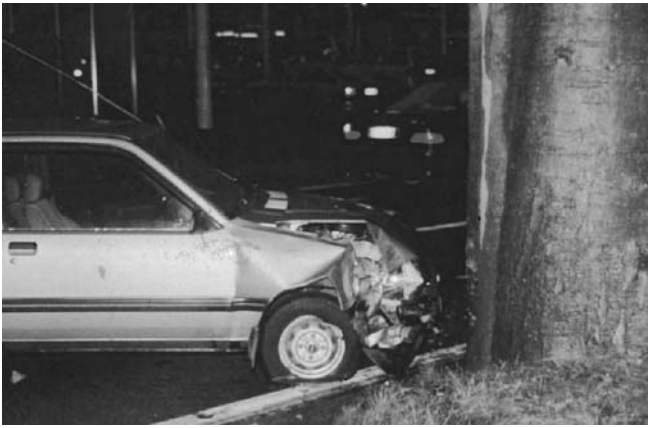
Fig. 1 Photograph of the case vehicle taken shortly after the collision with the tree. All of the damage to the vehicle is localized in the front passenger side
