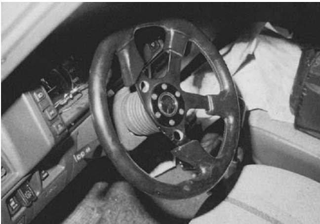
Fig. 2 Photograph of the interior of the case vehicle at the accident scene. Note the traces of blood near the bottom ( left ) hole in the steering wheel, and that the wheel is rotated approximately 90° counterclockwise
